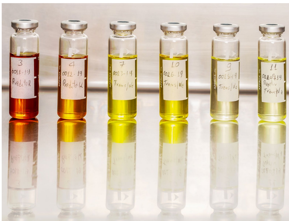
Fig. 2 Commercial PCB mixtures from transformers (source: Sonia Álvarez, SertinLab Ecuador)
